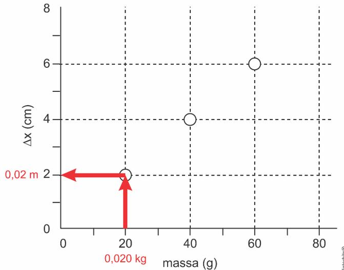
$$F_e = P \xrightarrow{\text{Lei de Hooke}} F_e = k \cdot \Delta x = m \cdot g \Rightarrow k = \frac{m \cdot g}{\Delta x} \Rightarrow k = \frac{0,020 \text{ kg} \cdot 10 \text{ m/s}^2}{0,02 \text{ m}} \therefore$$
